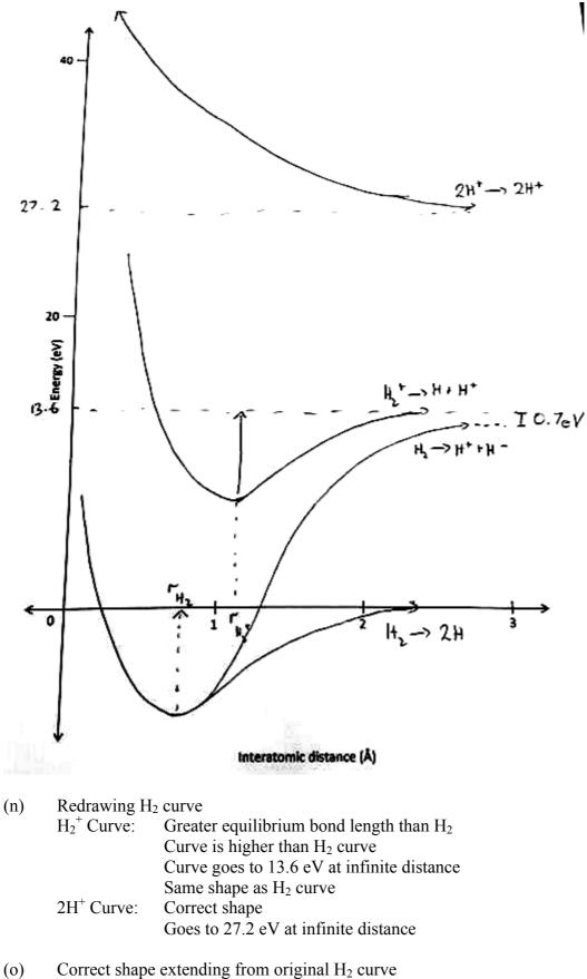
Correct shape extending from original  $H_2$  curve Goes to 13.6 - 0.7 = 12.9 eV at infinite distance
