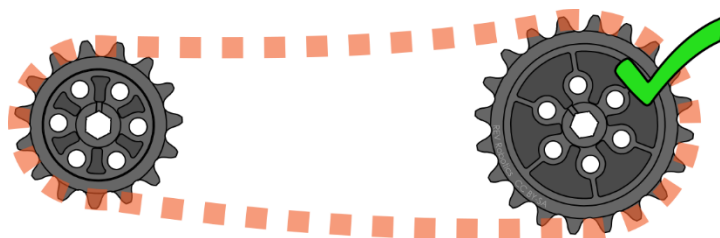
Figure 17: Correctly Spaced Sprockets (Chain Correctly Tensioned)
