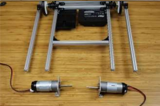
Use 8MM HEX CAP SCREWS to mount HD Hex Motor, 40:1 Gearbox to Bent HD Hex Motor Metal Bracket as shown.
