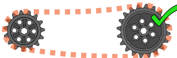
Figure 33: Correctly Spaced Sprockets (Chain Correctly Tensioned)
