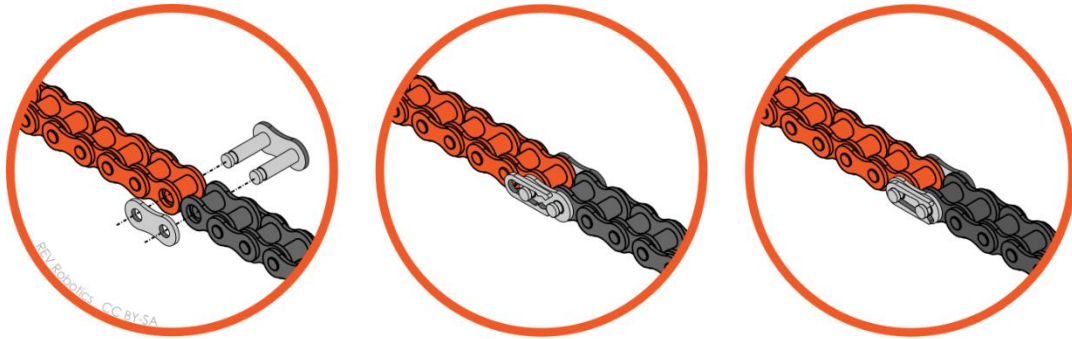
Figure 38: Master Link Assembly on Chain
