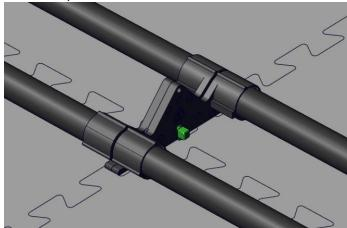
6. Layout a Horizontal Barrier Assembly on each end of the barrier. Each end should align with an Under Tile Plate.
