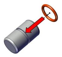
**Note:** Use your fingernail to press the Oring into the groove to ensure it stays in place during gameplay.
