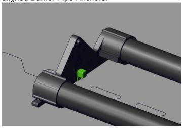
8. Add three additional cable ties to connect adjacent Anchors together.
