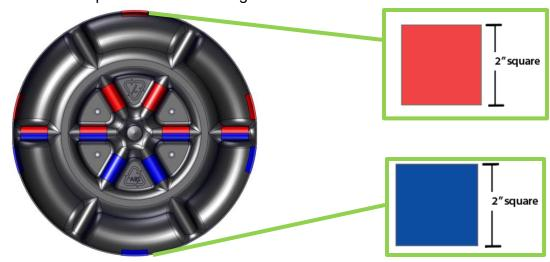
d. On adjacent red and blue sections, fold 2x2" square tape over the outer edge spaced 1" away from the center dividing line as shown.
