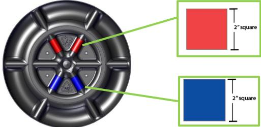
b. Divide the remaining with 1"x2" strips of red and blue tape to both the inner and outer rings.
