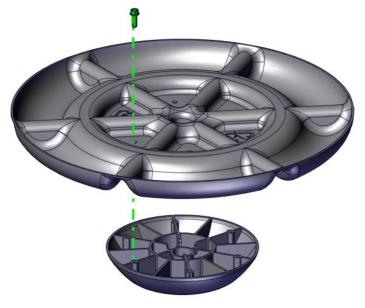
3. Loosely screw in the three remaining Base Fasteners.
