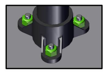
5. Tighten the Carousel Screws and Nuts until snug. Tighten just enough so that the flat heads of the screws sit flush with the top surface of the Platform.
