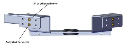
11. Install a pair of thumbscrews into the holes that correspond to the field perimeter type that you are using.
