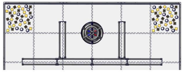
1. Select two pipes of the same length. Press a Barrier Pipe Anchor onto each end to make an assembly. A full field will have 3 Horizontal Barrier Assemblies and 2 Vertical Barrier Assemblies. Repeat this step for all 5 assemblies and set aside.
