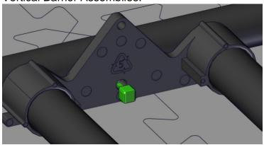
11. **Loosely** add a cable tie from the top hole of the Anchor on the Vertical Barriers (Locations #3,4) and wrap around the adjacent Horizontal Barrier Pipe.
