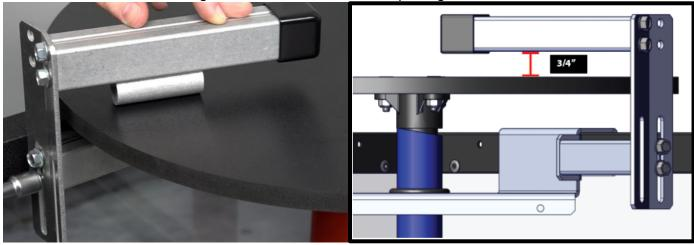
23. Add a Pinch Point Sticker to the Top Sweeper Arm by aligning the bottom of the sticker with the bottom of the Arm. Wrap the warning orange box onto the top surface. The text on the sticker should be viewable to the drive team in their respective red or blue alliance stations.
