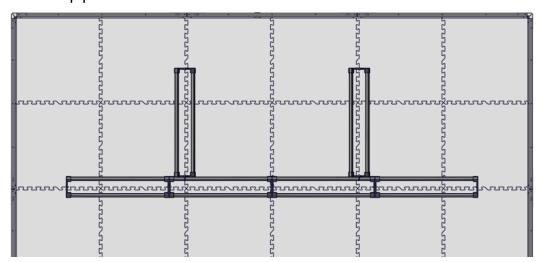
10. **Loosely** attach the cable ties on the Under Tile Plate (#1,2,3,4) to the adjacent Anchors on the Vertical Barrier Assemblies.
