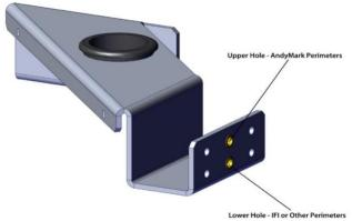
14. Install a pair of thumbscrews into the holes that correspond to the field perimeter type that you are using.
