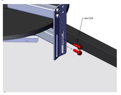
**Note:** These screws will need to be removed in order to disassemble the Carousel for transport and storage.
