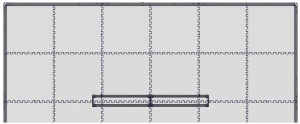
5. **Loosely** route the cable tie from the Under Tile Plate (#7) through the hole in the center Barrier Pipe Anchor.
