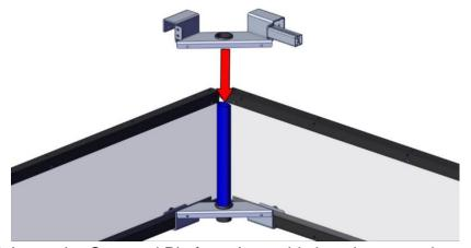
18. Insert the Carousel Platform Assembly into the open pipe.
