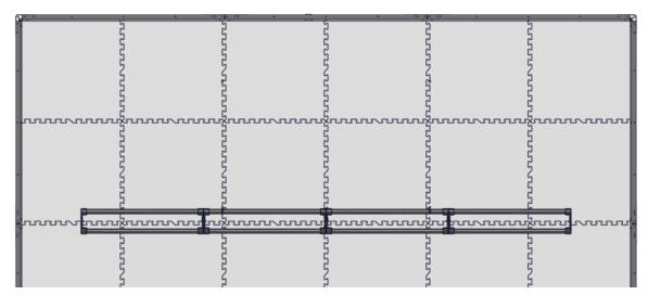
7. Loosely Route the cable ties from the corresponding Under Tile Plates (#5,6,8,9) through the aligned Barrier Pipe Anchors.
