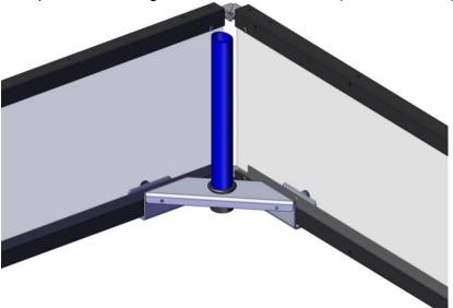
17. Using a twisting motion, slide the Top Bracket Assembly over the top of the Field Perimeter and onto the pipe. Secure to the field perimeter using the Bracket Hardware (thumb screws).
