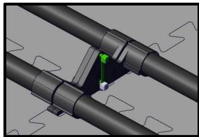
9. Layout the two Vertical Barrier Sections as shown. The anchor should be up against the horizontal pipe.
