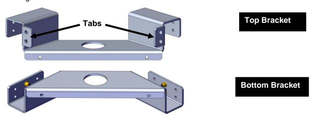
7. Insert a Grommet into the center hole in the Top Carousel Support Bracket.
