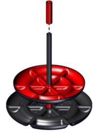
9. Add the same color Upper Tray (am-4493\_Red or Blue) to the assembly by pressing the center of the tray onto the pipe. This is Level 3.
