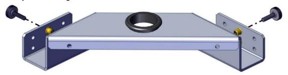
15. Locate the one Pipe Sleeve (Red or Blue) and a Pipe Bottom Cap (black). Push the Pipe Sleeve through the Bottom Carousel Support Bracket. Place the Bottom Cap underneath the Bracket and onto the Pipe Sleeve. Make sure the Bottom Cap is pushed all the way onto the bottom of the pipe. The Bottom Cap sits on the floor.
