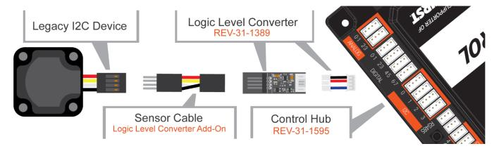
Figure 7: Connecting a Legacy 5V Sensor to a Control Hub
