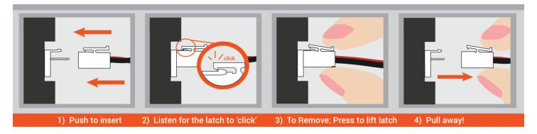
Figure 1: How to Use a JST VH Cable
