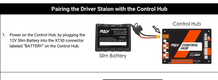
The Control Hub is ready to pair with the Driver Station when the LED turns green. Note: the light blinks blue every ~5 seconds to indicate that the Control Hub is healthy.
