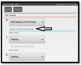
8. Repeat the process for "Port 1" and name the motor "right\_drive".
