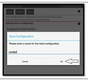
14. You now have an active configuration called "miniBot". Press the Android back button to return to the Driver Station page.
