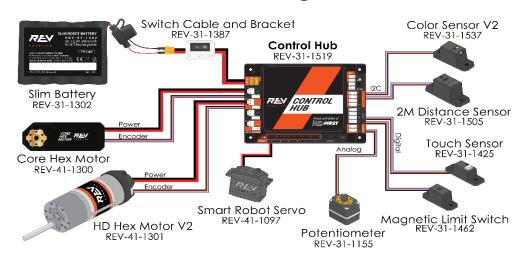
**Figure 3: System Wiring Diagram**
