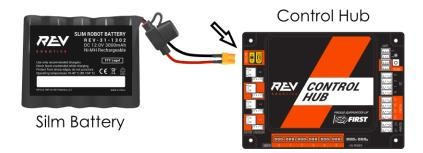
The Control Hub is ready to connect with a PC when the LED turns green. Note: the light blinks blue every ~5 seconds to indicate that the Control Hub is healthy.
