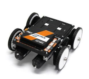
Figure 4: The miniBot is a Simple 2-Motor Robot
