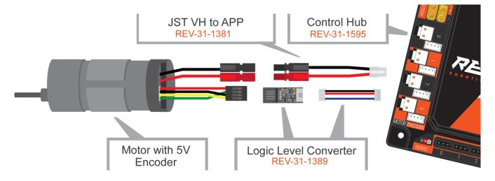
Figure 6: Connecting a Motor with 5V Encoder to a Control Hub
