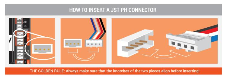
Figure 2: How to Use a JST PH Cable
