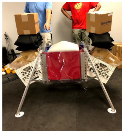
(First Load to Failure test, 207lbs held by each side of the lander)
