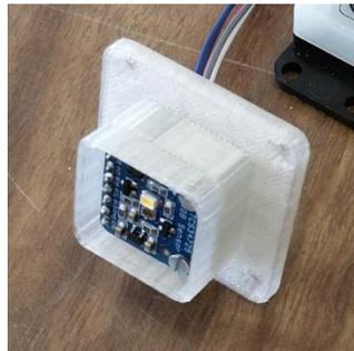
Figure 35 - A simple open-faced housing that secures the Sensor and can be mounted to a Robot.
