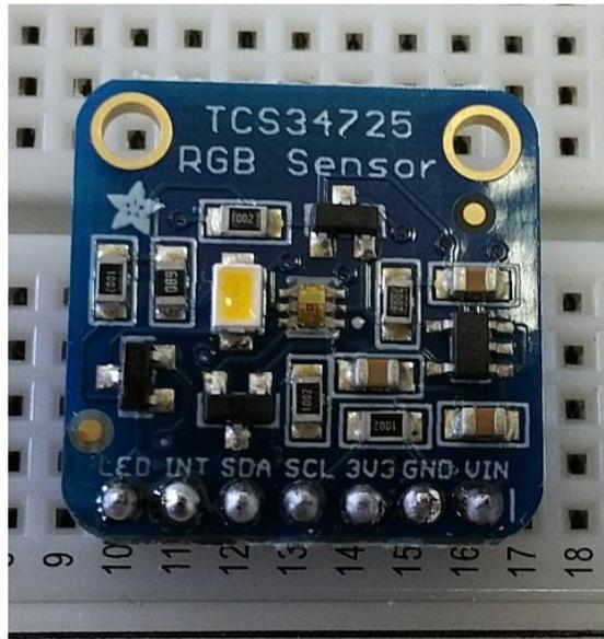
Figure 11 – The Sensor has 7 pins (LED, INT, SDA, SCL, 3V3, GND and VIN).
