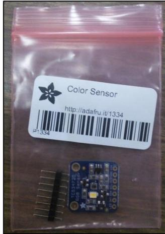
Figure 1 - The AdaFruit RGB Sensor is sold as a board without any protective case or a connector cable.
