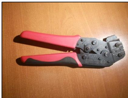
**Figure 16 - Molex terminal crimping tool.**
