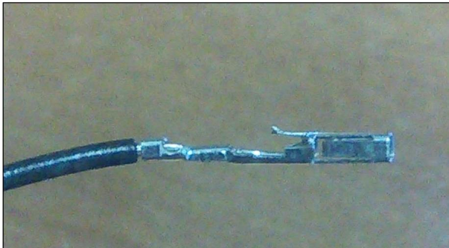
**Figure 18 - Crimp a terminal onto one end of the wire.**
