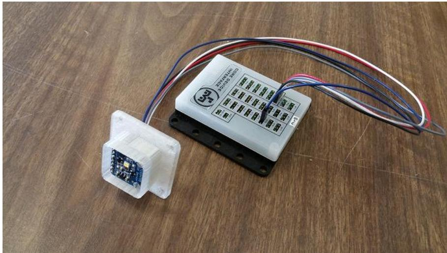
Figure 2 – This guide shows to assemble the Sensor into a mountable housing & how to create a connector cable
