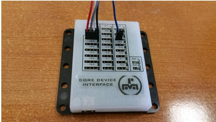
Figure 28 - Connect LED pin to a digital signal pin on the CDI module if you want to control the LED with that port.
