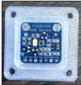
**Figure 39 - Secure the Sensor using two #2 wood screws (1/2" in length).**
