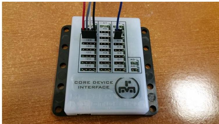
Figure 41 - Plug the 4-circuit and 2-circuit (1-wire) housings into an I2C port and digital port respectively.
