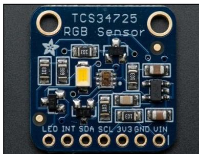
Figure 4 - The Sensor has 7 pins.
