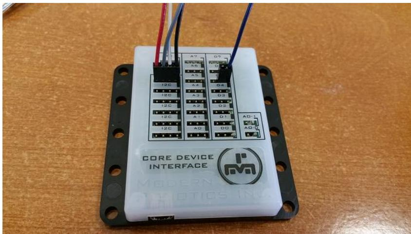
Figure 29 - Connect LED pin to a ground pin on the CDI module if you want to keep the LED turned off.
