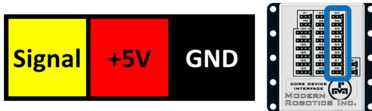
Figure 27 - Layout of digital port on CDI module.
