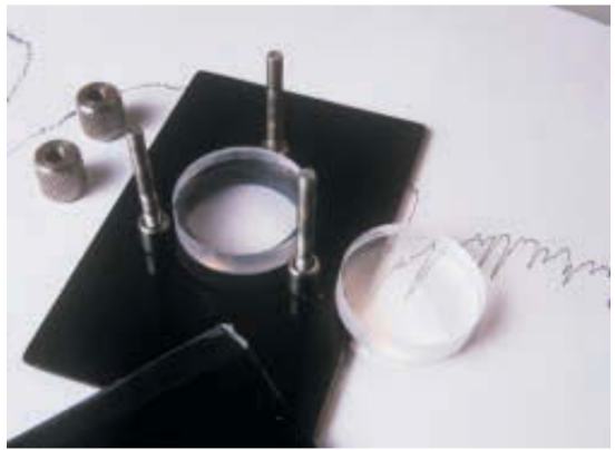
salt plate (NaCl) transparent to IR radiation
