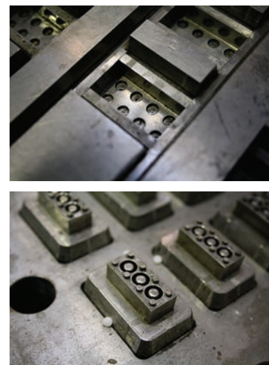
FIGURE 26-32 Injection molding of thermoplastic polymers (a) Upper and lower sides of the molds used to produce Lego blocks. (b) Blocks produced from the injection molding process.
