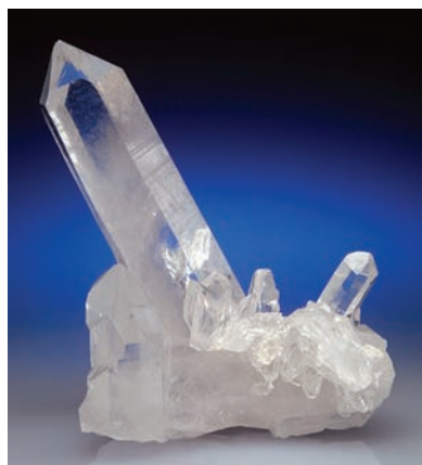
FIGURE 1-3 Quartz crystal Quartz (silicon dioxide) is the silicon analog of carbon dioxide. Whereas carbon dioxide is gaseous, silicon dioxide is a solid.
