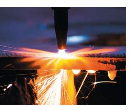
An oxygen—acetylene flame is hot enough to melt steel for welding. A cutting torch uses an extra jet of oxygen to burn away hot steel.
