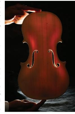
The acoustic properties of cellulose have never been surpassed by other substances. Here, a luthier holds a spruce front plate up to a light to show how the thickness is carefully graduated to enhance a pleasing sound.
