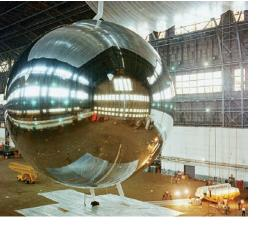
The Echo satellite was a 41-meter balloon made of metallized Mylar® film. It was launched in 1964 to reflect radio waves for intercontinental telephone, radio, and television. Echo was easily visible to the unaided eye as it orbited the Earth until 1969, when it reentered the atmosphere and burned up.
