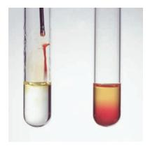
When a solution of bromine (redbrown) is added to cyclohexene, the bromine color quickly disappears because bromine adds across the double bond. When bromine is added to cyclohexane (at right), the color persists because no reaction occurs.
