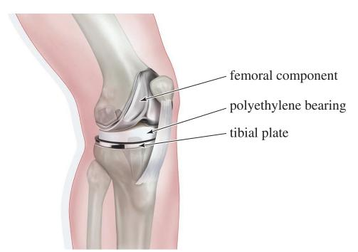
▲ Polyethylene provides a self-lubricating surface for movement of the metal parts of an artificial knee replacement. The highly cross-linked polyethylene used in these implants is fabricated to be exceptionally tough: It wears only about 0.1 mm per year. Polyethylene is compatible with the human body, and in most cases, it does not cause a foreign body reaction even after years of constant movement in the joint.
