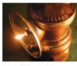
A miner's carbide lamp. Water in the upper chamber slowly drips onto calcium carbide in the lower chamber, generating acetylene.
