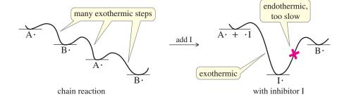
"Butylated hydroxyanisole" (BHA) is often added to foods as an antioxidant. It stops oxidation by reacting with radical intermediates to form a relatively stable free-radical intermediate (BHA radical). The BHA radical can react with a second free radical to form an even more stable quinone with all its electrons paired.
