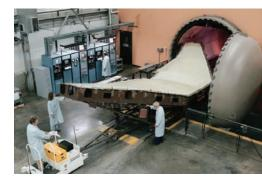
Workers guide the skin for the tail of a Harrier II jet into an autoclave where its layers of epoxy-coated carbon-fiber cloth will be bonded and cured under heat and pressure. The carbon-epoxy composite is used to make aircraft parts that are as strong as steel but as light as aluminum. This second epoxide reacts with another molecule of bisphenol A. Each molecule of bisphenol A can also react with two molecules of epichlorohydrin.
