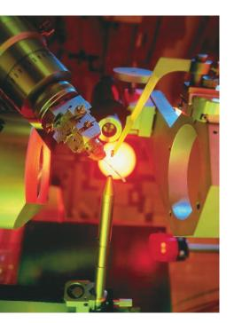
Tertiary structures of proteins are determined by X-ray crystallography. A single crystal of the protein is bombarded with X rays, whose wavelengths are appropriate to be diffracted by the regular atomic spacings in the crystal. A computer then determines the locations of the atoms in the crystal.
