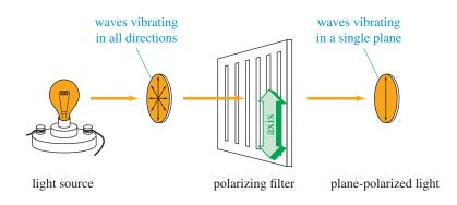
FIGURE 5-11 Function of a polarizing filter. The waves of plane-polarized light vibrate
