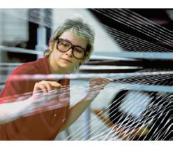
Production of continuous-filament nylon tire cord.
