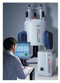
Photo of a 300-MHz NMR spectrometer. The metal container at the back contains the superconducting magnet, cooled by a liquid helium bath. The electronics used to control the spectrometer and to calculate spectra are at right.
