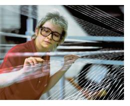
Production of continuous-filament nylon tire cord.
