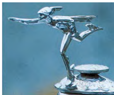
Chromium is often used to plate bumpers and hood ornaments, such as this statue of Mercury found on a 1929 Buick.
