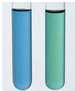
The blue solution contains \text{Cr}^{2+} ions, and the green solution contains \text{Cr}^{3+} ions.
