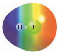
FIGURE 8.4 An electrostatic potential map of HF. Red indicates the most electron-rich area (the fluorine atom) and blue indicates the most electron-poor region (the hydrogen atom).
