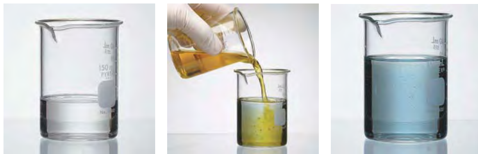
When potassium dichromate reacts with ethanol, a blue-violet solution containing \text{Cr}^{3+} is formed.
