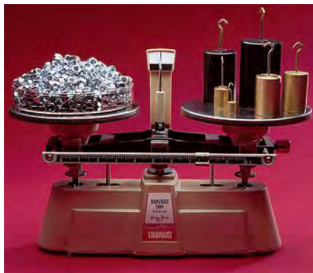
It is much easier to weigh out 600 hex nuts than count them one by one.
