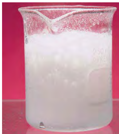
Hydrochloric acid reacts with solid sodium hydrogen carbonate to produce gaseous carbon dioxide.
