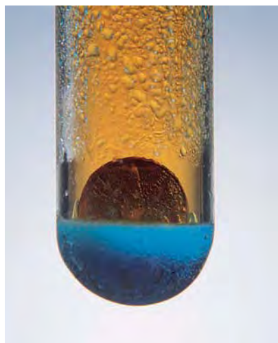
A copper penny reacts with nitric acid to produce NO gas, which is immediately oxidized in air to brown NO_2 .
