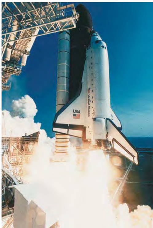
The main engines in the space shuttle Endeavour use hydrogen and oxygen as fuel.
