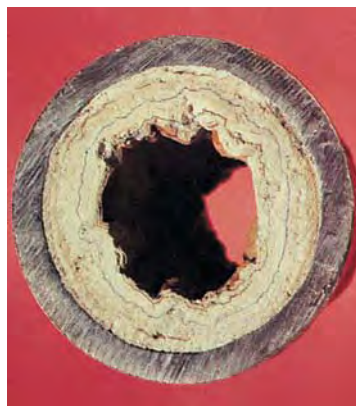
FIGURE 11.8 A pipe with accumulated mineral deposits. The cross section clearly indicates the reduction in pipe capacity.
