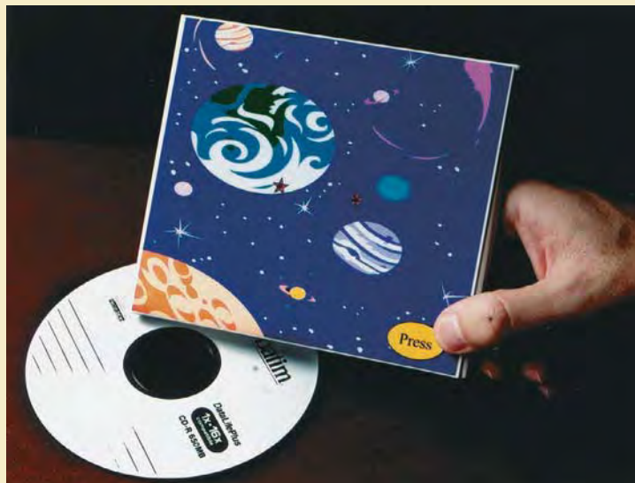
A CD case with an ultrathin battery that can be “printed” on packages like ink.
