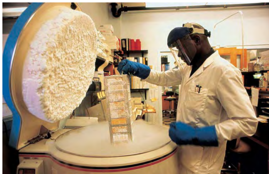
At the Centers for Disease Control and Prevention in Atlanta, Georgia, a worker checks samples stored in a liquid nitrogen tank.
