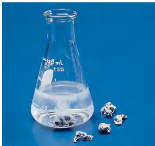
The reaction of zinc with hydrochloric acid to produce bubbles of hydrogen gas.
