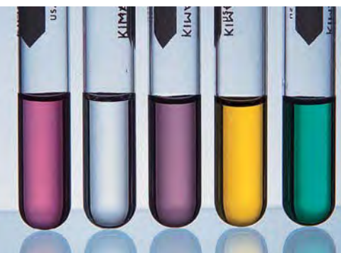
(from left to right) Aqueous solutions containing the metal ions \text{Co}^{2+} , \text{Mn}^{2+} , \text{Cr}^{3+} , \text{Fe}^{3+} , and \text{Ni}^{2+} .
