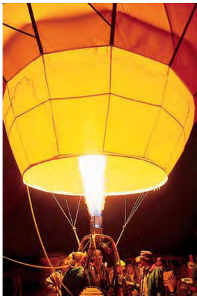
A propane burner is used to heat the air in a hot-air balloon.
