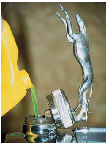
The addition of antifreeze lowers the freezing point of water in a car's radiator.
