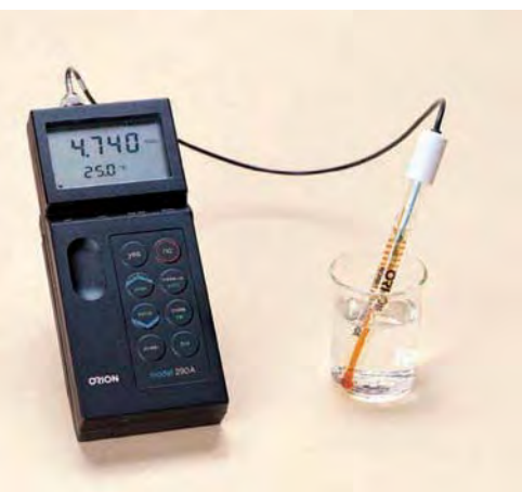
A digital pH meter shows the pH of the buffered solution to be 4.740.
