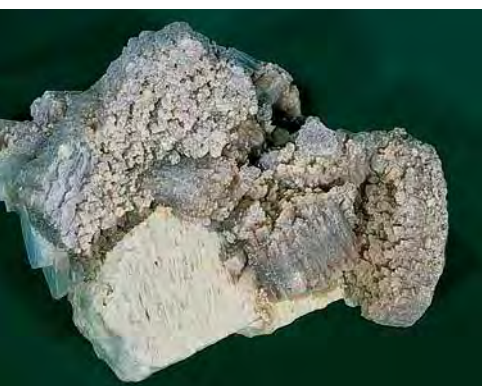
FIGURE 19.4 Lepidolite is composed mainly of lithium, aluminum, silicon, and oxygen, but it also contains significant amounts of rubidium and cesium.
