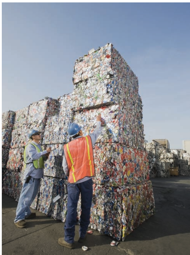
FIGURE SA7.2 Recycling aluminum cans. Converting old aluminum cans into new aluminum cans requires only 6 percent of the energy used to convert aluminum ore from a mine into new aluminum cans. (Erik Isakson/age fotostock)
