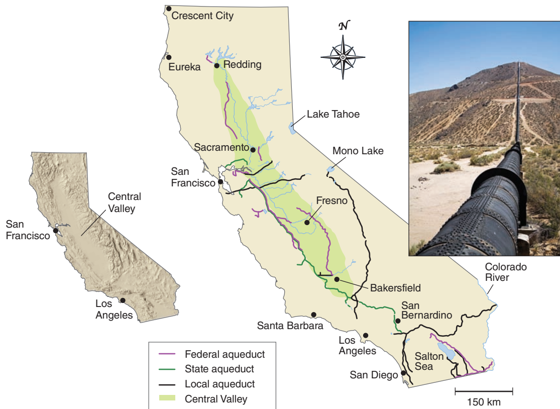
FIGURE SA4.1 Water distribution in California. To supply water to the agricultural areas in the Central Valley and to supply drinking water to municipalities, the state has developed an elaborate system of aqueducts. These aqueducts consist of both open canals and pipes laid above or below the ground. (Jim West/The Image Works)
