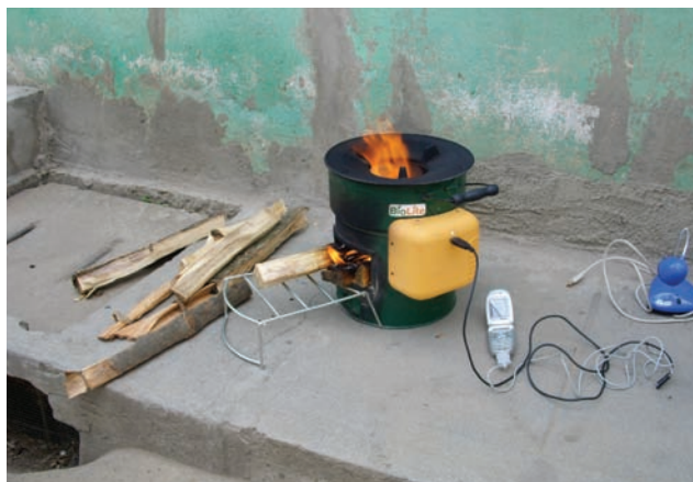
BioLite cookstove. This small stove, and others like it, has the potential to reduce the amount of firewood needed to cook a meal, and lower the amount of indoor air pollution emitted as well. (Jonathan den Hartog; courtesy of Jonathan Cedar, www.BioLiteStove.com )
