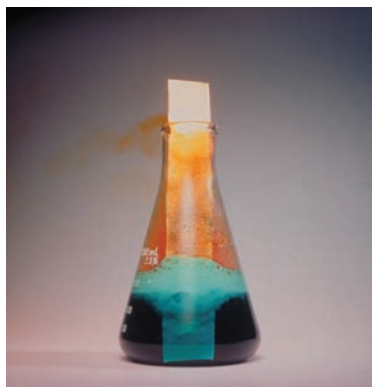
FIGURE 9.11 When copper metal is immersed in concentrated nitric acid, the copper is oxidized and an aqueous solution of blue copper(II) nitrate forms. In addition, some of the nitrate ion is reduced to brown gaseous nitrogen dioxide, which bubbles off.
