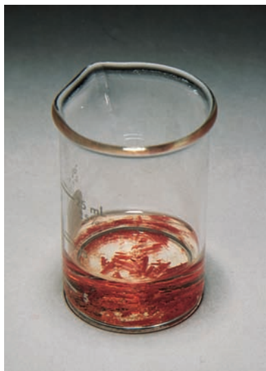
FIGURE 16.1 The beaker contains an aqueous solution of K_2PtCl_4 , a substance used as a starting material in the synthesis of anticancer drugs. It is loosely covered to keep out dust and allowed to stand. As the water evaporates, the solution becomes saturated and deposits solid K_2PtCl_4 in the form of long, needle-like red crystals.
