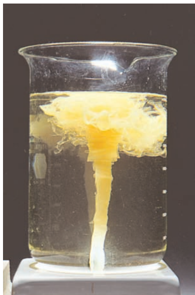
FIGURE 16.14 The “orange tornado” is a striking demonstration of the effects of complex ions on solubility. A solution is prepared with an excess of \text{I}^-(aq) over \text{Hg}^{2+}(aq) so that the \text{Hg}^{2+} is complexed as \text{HgI}_3^- and \text{HgI}_4^{2-} . A magnetic stirrer is used to create a vortex in the solution. Addition of a solution containing \text{Hg}^{2+} down the center of the vortex then causes the orange solid \text{HgI}_2 to form in a layer at the edges of the vortex, giving the tornado effect.
