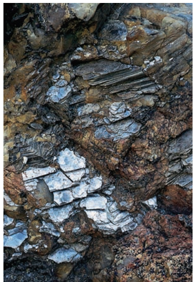
FIGURE 22.5 Naturally occurring muscovite mica. The mechanical properties of crystals of mica are quite anisotropic. Thin sheets can be peeled off a crystal of mica by hand, but the sheets resist stresses in other directions more strongly. Transparent, thin sheets of mica, sometimes called isinglass, have been used for heat-resistant windows in stoves or in place of window glass.
