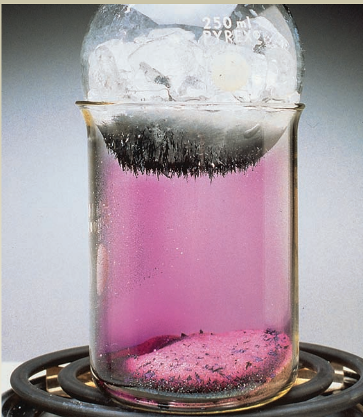
Solid iodine is converted directly to a vapor (sublimes) when warmed. Here, purple iodine vapor is redeposited as a solid on the cooler upper surfaces of the vessel.
