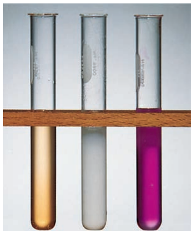
FIGURE 16.16 Zinc hydroxide is insoluble in water (center) but dissolves readily in acid (left) and base (right). The indicator used is bromocresol red, which turns from red to yellow in acidic solution.
