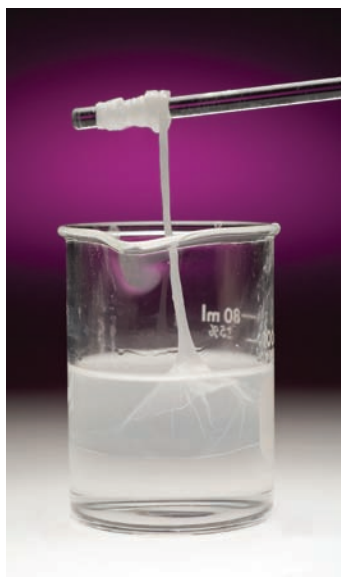
FIGURE 23.5 Hexamethylenediamine is dissolved in water (lower layer), and adipyl chloride, a derivative of adipic acid, is dissolved in hexane (upper layer). At the interface between the layers, nylon forms and is drawn out onto the stirring bar.
