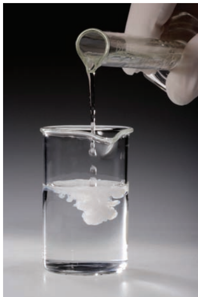
FIGURE 11.6 A solution of potassium sulfate is being added to one of barium chloride. A cloud of white solid barium sulfate is formed; the potassium chloride remains in solution.
