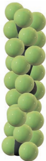
FIGURE 23.7 A model of the molecular structure of Teflon shows that the fluorine atoms shield the carbon chain very effectively. Note that the chain must twist to accommodate the bulk of the fluorine atoms, completing a full spiral every 26 C atoms along the chain.
