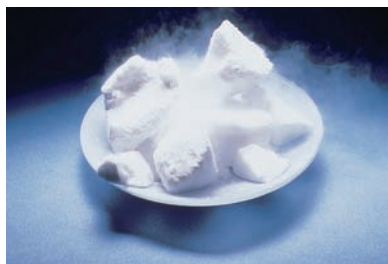
FIGURE 10.25 Sublimation of solid carbon dioxide (dry ice). The white clouds are drops of water vapor (moisture in the air) that condense at the low temperatures near the solid surface. Gaseous carbon dioxide itself is transparent.
