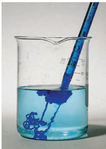
FIGURE 23.4 Filter paper (cellulose) will dissolve in a concentrated ammonia solution containing [\text{Cu}(\text{NH}_3)_4]^{2+} ions. When the solution is extruded into aqueous sulfuric acid, a dark blue thread of rayon (regenerated cellulose) precipitates.
