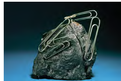
▲ FIGURE 23.6 A permanent magnet. Permanent magnets are made from ferromagnetic and ferrimagnetic materials.
