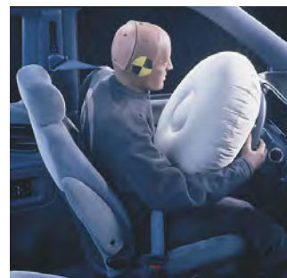
▲ FIGURE 3.7 Decomposition of sodium azide, \text{NaN}_3(s) , is used to inflate automobile air bags.
