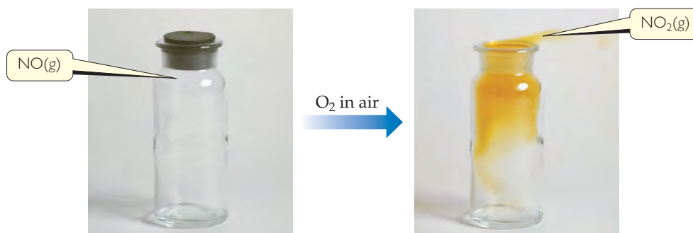
▲ FIGURE 22.25 Formation of \text{NO}_2(\text{g}) as \text{NO}(\text{g}) combines with \text{O}_2(\text{g}) in the air.
