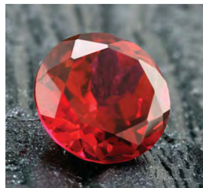
\blacktriangleright FIGURE 12.25 Brittleness and faceting in ionic crystals. (a) When a shear stress is applied to an ionic solid, the crystal separates along a plane of atoms as shown here. (b) This property of ionic crystals is used to facet gemstones, such as rubies.
