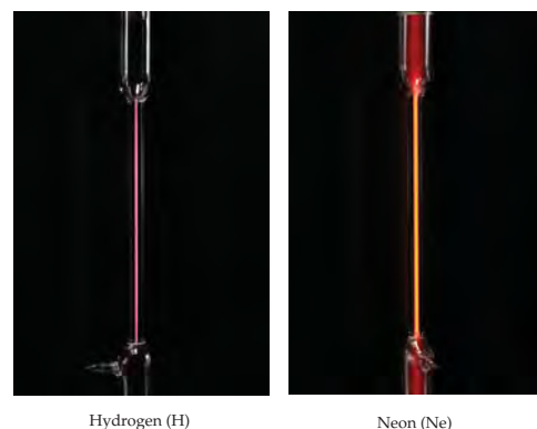
▲ FIGURE 6.10 Atomic emission of hydrogen and neon. Different gases emit light of different characteristic colors when an electric current is passed through them.
