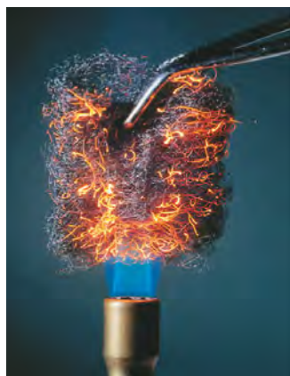
Steel wool heated in air (about 20% O_2 ) glows red-hot but oxidizes to Fe_2O_3 slowly
