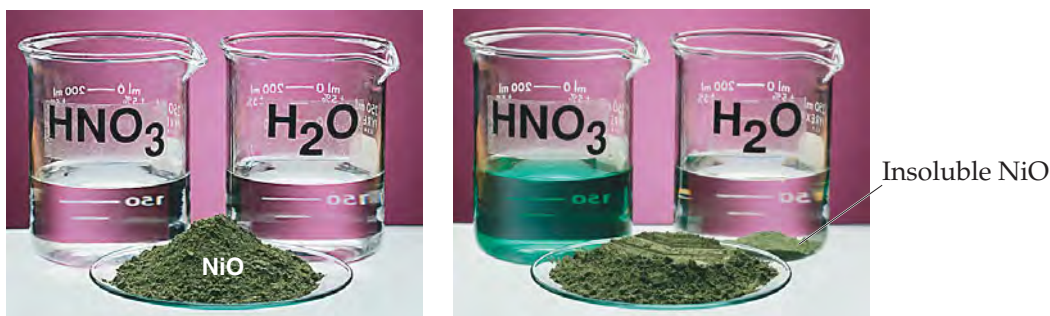
► FIGURE 7.15 Metal oxides react with acids. NiO does not dissolve in water but does react with nitric acid (HNO 3 ) to give a green solution of Ni(NO 3 ) 2 .
