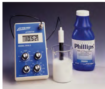
▲ FIGURE 16.6 A digital pH meter. The device is a millivoltmeter, and the electrodes immersed in a solution produce a voltage that depends on the pH of the solution.
