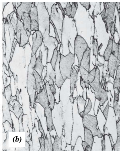
Figure 7.11 Alteration of the grain structure of a polycrystalline metal as a result of plastic deformation. (a) Before deformation the grains are equiaxed. (b) The deformation has produced elongated grains. 170 \times . (From W. G. Moffatt, G. W. Pearsall, and J. Wulff, The Structure and Properties of Materials , Vol. I, Structure , p. 140. Copyright © 1964 by John Wiley & Sons, New York.)
