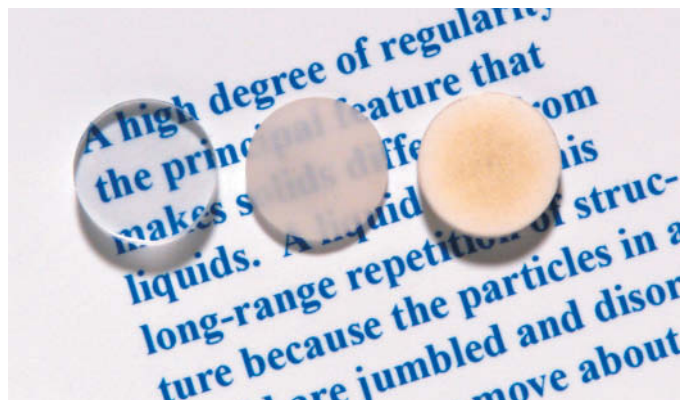
Figure 21.10 The light transmittance of three aluminum oxide specimens. From left to right; single-crystal material (sapphire), which is transparent; a polycrystalline and fully dense (nonporous) material, which is translucent; and a polycrystalline material that contains approximately 5% porosity, which is opaque. (Specimen preparation, P. A. Lessing.)
