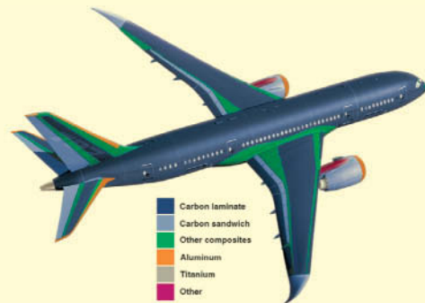
Figure 16.20 Locations of the various material types used in the Boeing 787 Dreamliner.
