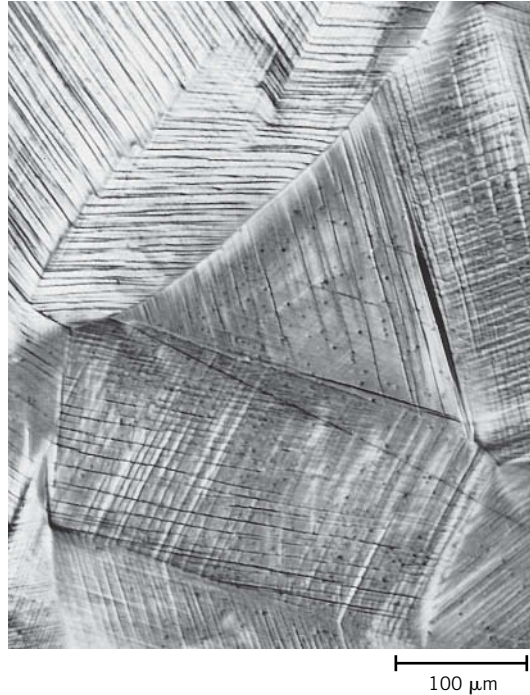
Figure 7.10 Slip lines on the surface of a polycrystalline specimen of copper that was polished and subsequently deformed. 173 \times . [Photomicrograph courtesy of C. Brady, National Bureau of Standards (now the National Institute of Standards and Technology, Gaithersburg, MD).]
