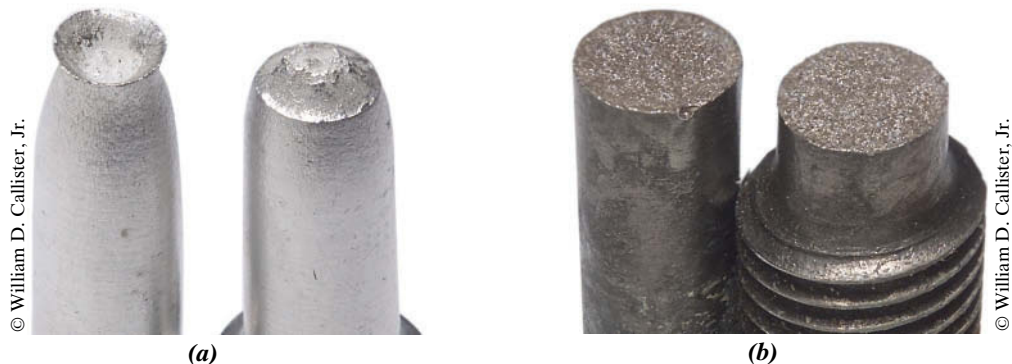
Figure 8.3 (a) Cup-and-cone fracture in aluminum. (b) Brittle fracture in a mild steel.
