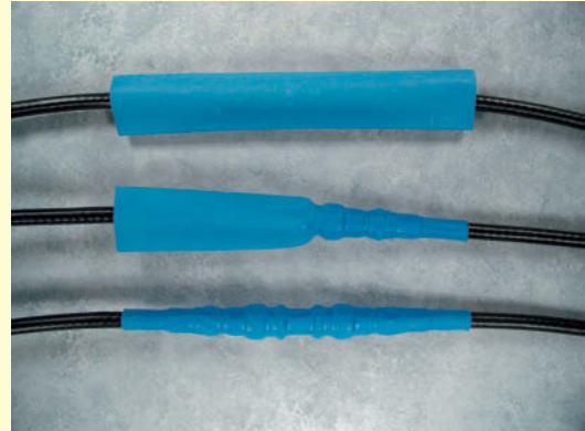
Top: An electrical connection positioned within a section of as-received polymer shrink-tubing. Center, Bottom: Application of heat to the tubing caused its diameter to shrink. In this constricted form, the polymer tubing stabilizes the connection and provides electrical insulation. (Photograph courtesy of Insulation Products Corporation.)
